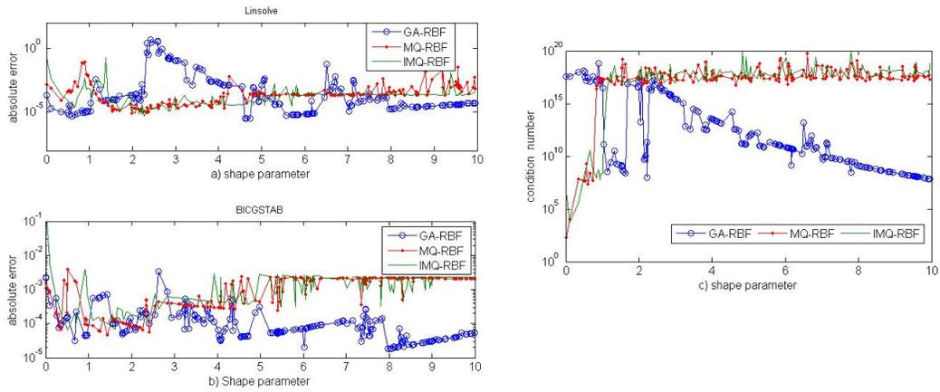
FIGURE 2. a) Absolute error vs. shape parameter. b) Absolute error when Using Bicgstab method. c) Condition number vs. shape parameter.
